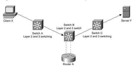
Figure 2-2 Flow of intersubnet traffic with Layer 3 switches.
