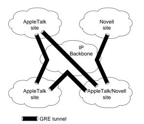
Figure 2-10 Using a single protocol backbone.
