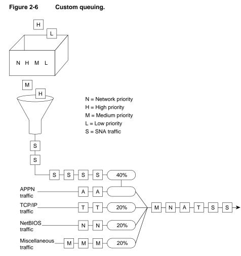
Custom queuing prioritizes multiprotocol traffic. A maximum of 16 queues can be built with custom queuing. Each queue is serviced sequentially until the number of bytes sent exceeds the configurable byte count or the queue is empty. One important function of custom queuing is that if SNA traffic uses only 20 percent of the link, the remaining 20 percent allocated to SNA can be shared by the other traffic.
