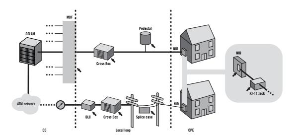
figure 9 Physical layer for test access points
