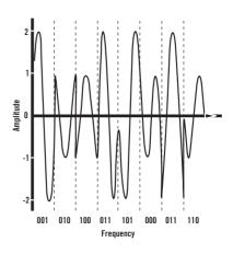
figure 6 Example of QAM encoding
