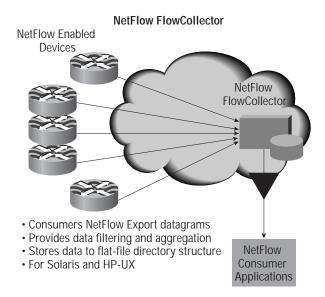
The FlowCollector passively listens to specified UDP ports to receive and process exported NetFlow datagrams. The FlowCollector application provides a high performance, easy-to-use solution that scales to accommodate consumption of NetFlow Export data from multiple devices in order to support key flow-consumer applications including accounting, billing, and network planning/monitoring.
